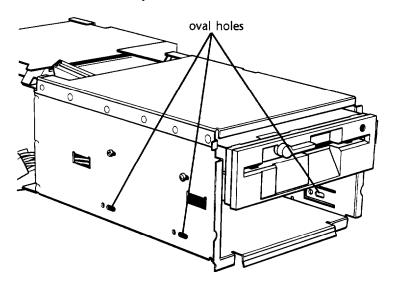
3. Insert the drive in the lower drive bay and slide it toward the back of the subassembly. Watch the oval holes on the side of the drive bay so you can see when the holes on the drive are positioned in the middle of them.
